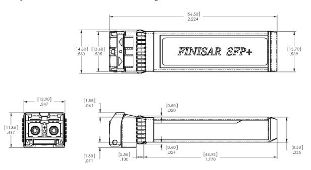
Figure 5. FTLX1371D3BCL Mechanical Dimensions
