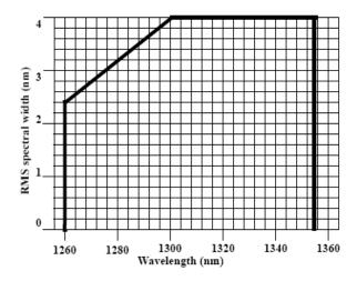
**Transmitter Maximum RMS Spectral Width** Figure 3.
